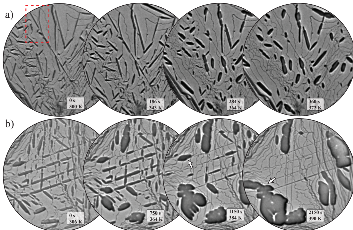
Figure 7.3: Two examples for the transformation of the \alpha -phase needles into the \beta -phase, which is characterized by increasingly compact island shapes. Annealing times are defined as the time lapse from the start of the temperature increase. The curved lines represent step(bunche)s and the straight lines show the intersection of glide planes with the (111)-surface and are thus oriented along close packed azimuth directions. The experiment in the top row ( a ) started at a lower initial BDA coverage, and features a shorter anneal at a lower final temperature as compared to the experiment in the bottom row ( b ). The longer annealing at a higher temperature results in ripening of the \beta -phase domains and therefore a lower island density. The dashed box in the first image indicates the area presented in detail in Fig. 7.4. Top row: FoV 10\ \mu\text{m} , start voltage 3\ \text{V} , bottom row: FoV 6\ \mu\text{m} , start voltage 2.7\ \text{V} .
